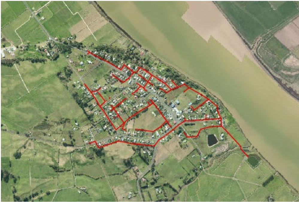
Figure 6.4.2.2: The extent of Te Kopuru’s wastewater network.
