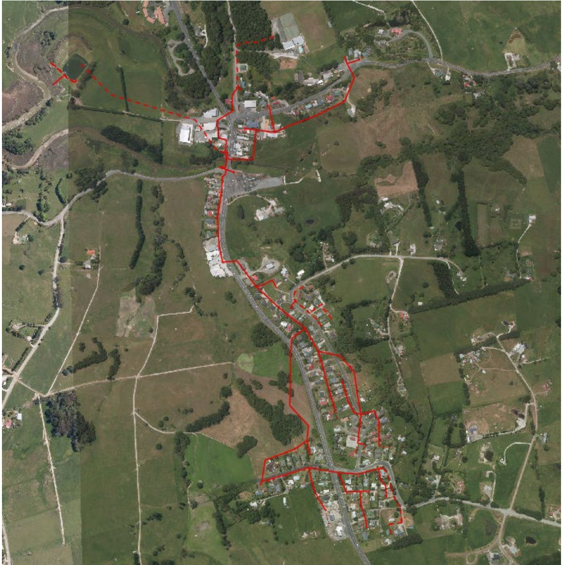
Figure 6.4.2.5: The extent of Kaiwaka's wastewater network.
