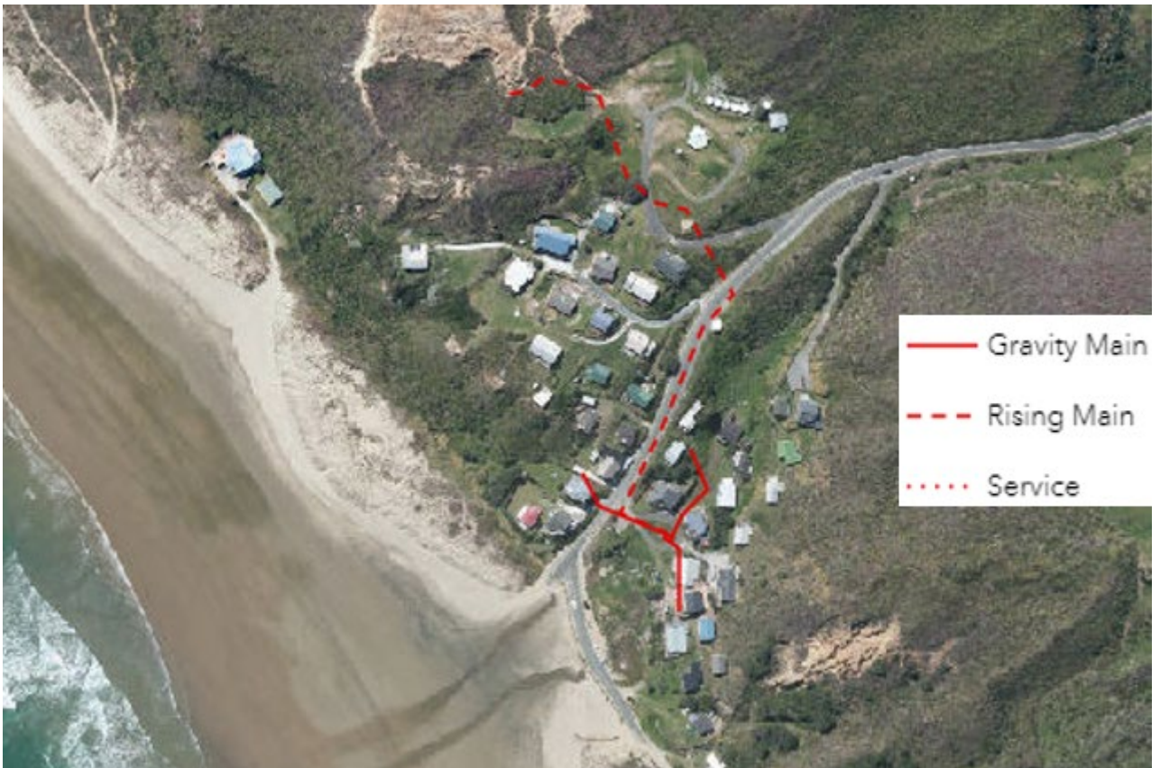
Figure 6.4.2.3: The extent of Glinks Gully’s wastewater network.
